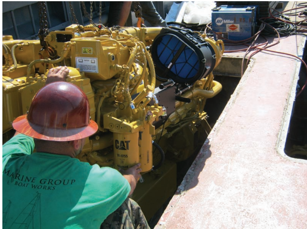
A worker at Marine Group Boat Works in San Diego guides an engine through the deck of the Piper Inness .
