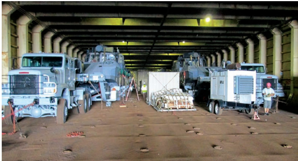
The Mark V boats, along with their tractors and trailers, are lashed in the covered area of the ATB.
